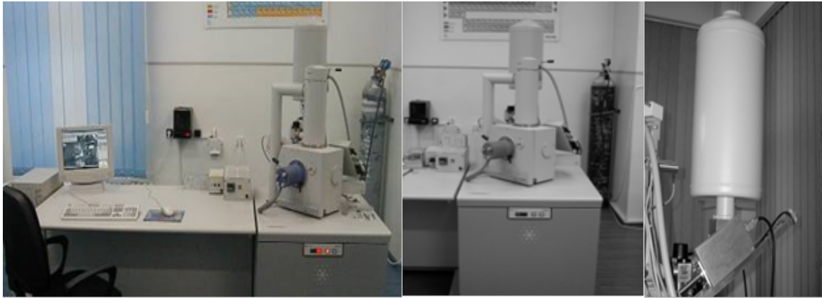
Figure 5.4 Philips scanning electron microscope model ESEM XL 30 TMP, equipped with an EDAX energy spectrometer
