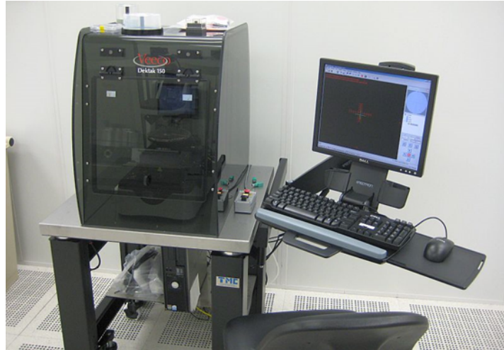
Figure 4.3 The device used for roughness determination
